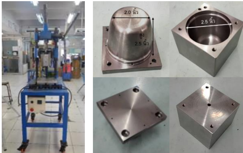
Figure 1 The vertical ram extruder machine for the conical plant pots.
